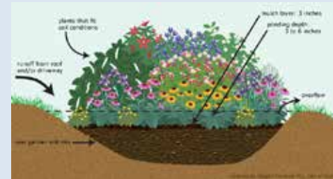
Rain garden diagram (Source: City of Durham)
