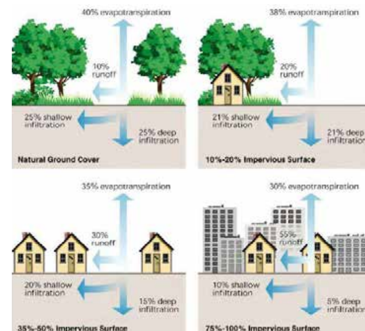
The diagram illustrates how increasing the amount of impervious surfaces increases the amount of runoff. (Source: Federal Interagency SRWG)
